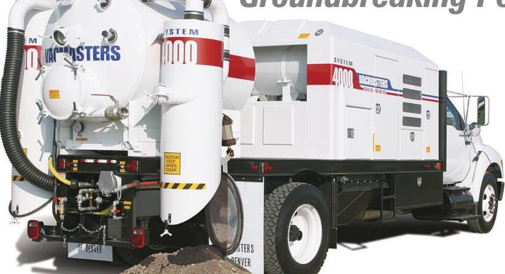
The SYSTEM 4000 is the workhorse of vacuum excavators, with the brute force to dig deep down with air, exposing utilities in even the hardest soils without harming them. Now you can dig faster, easier, and safer in soil that's hard, wet, sunbaked, or compact, including ground frost.
